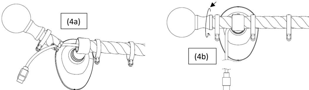
5. Mount the control box to the wall behind the curtain stack, attach the power pendant below the control box, and install the weighted wands.
