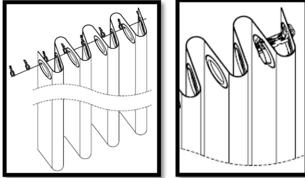
2. Snap the driver clip onto the first two grommets. Make sure to have pilot end on the first grommet, and the string from the clip comes out the slit of the supporting end.
