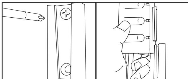
Figure 2.5.1 - Attach sensor box to wall
