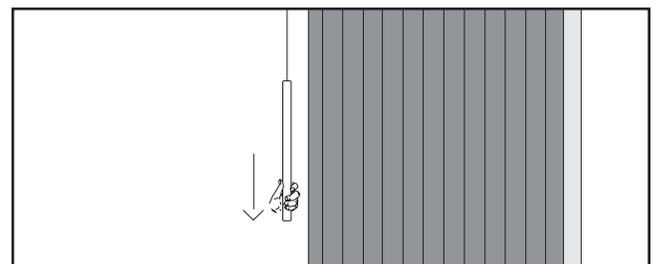
Figure 20 - Pull down and release Pendant
