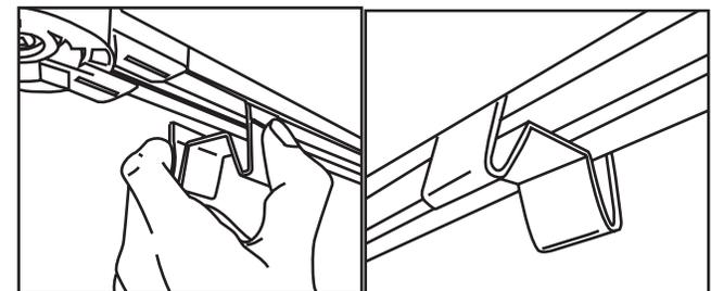
Figure 21 - Use clips to hold up track.
