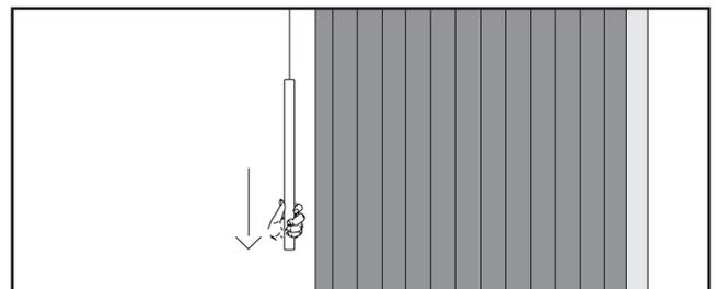
Figure 24 - Pull down and release Pendant
