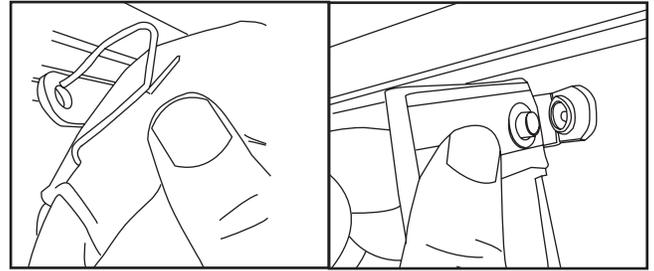
Figure 2.6.1 - Hook or snap drapery onto carriers
