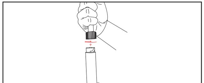
Figure 2.8.3.1 - Screw the Pendant onto the Cord
