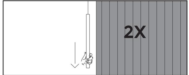
Figure 25 - Pull down and release Pendant
