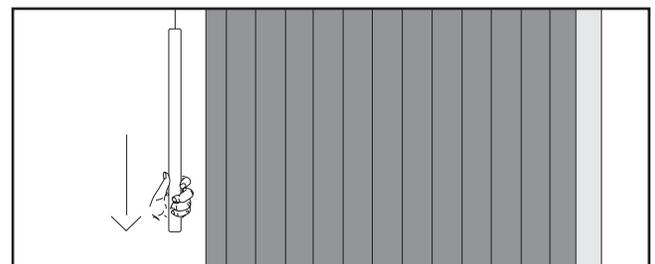
Figure 32 - Pull down and release Pendant once
