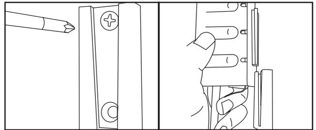
Figure 2.5.1 - Attach sensor box to wall
