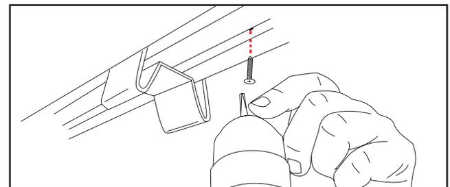
Figure 21 - Permanently secure track to recessed extrusion.
